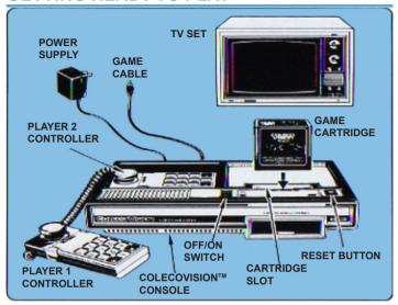
Make sure the COLECOVISION console is connected to your TV. Make sure power supply is plugged into the console. Then plug power supply into your AC outlet.
